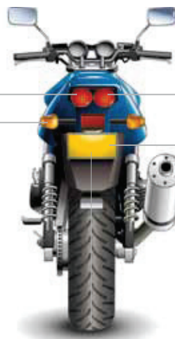
R5W W3W W5W T4W H6W W21/5W P21/5W Rear parking lights
